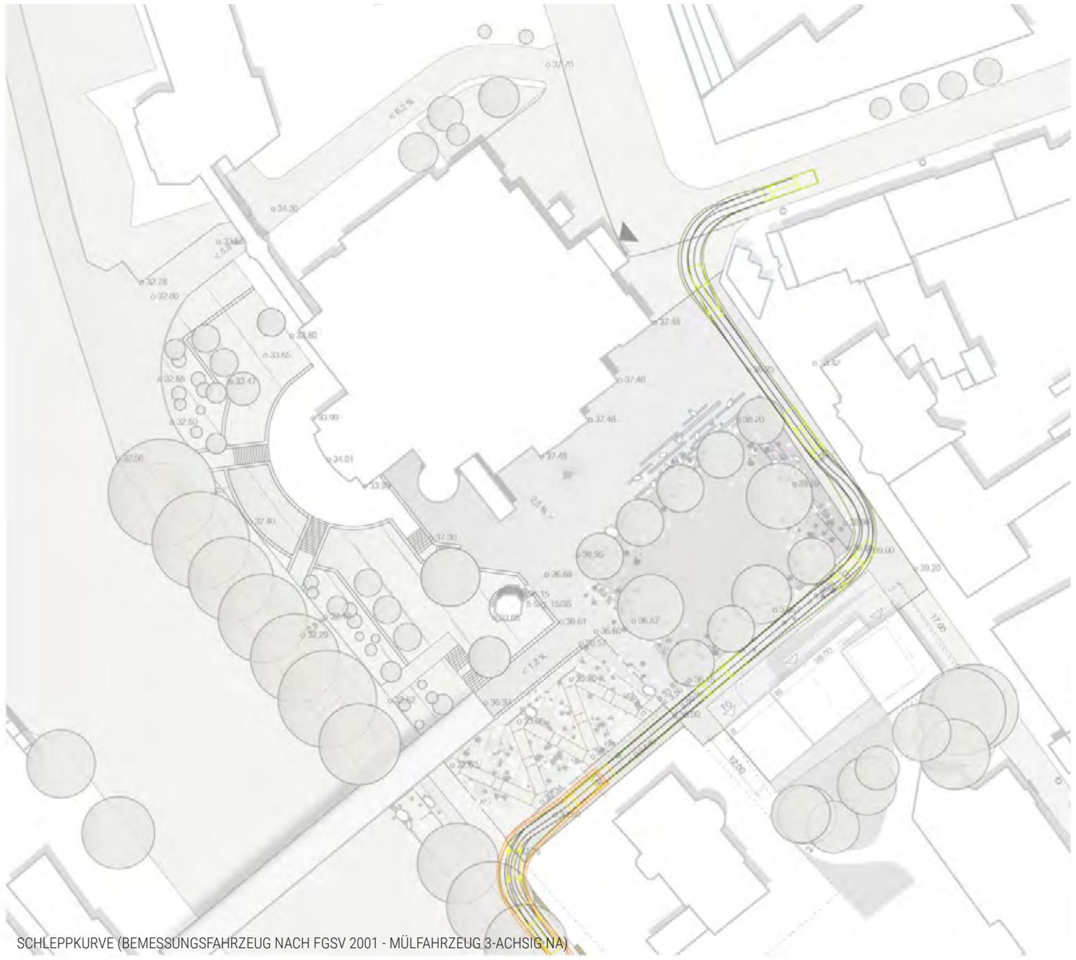
SCHLEPPKURVE (BEMESSUNGSFAHRZEUG NACH FGSV 2001 - MÜLFahrZEUG 3-ACHSIG NA)
